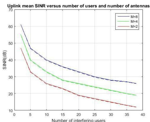
Fig. (5) Uplink mean SINR versus number of users and number of antennas
