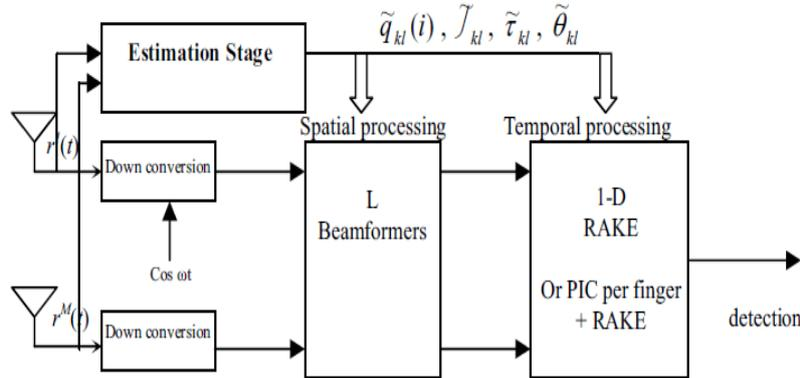
Fig.(1) 2D-RAKE receiver
